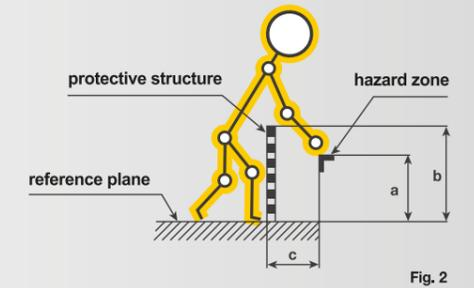
In the following table (relevant to high risk) the protective structures with a lower height of 1000 mm, are not mentioned because they do not limit enough, the movement of the body.
