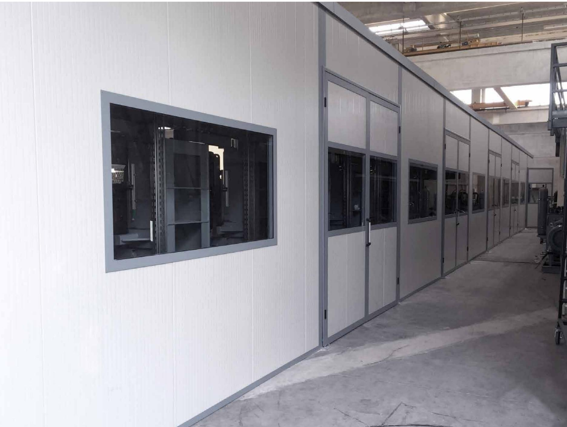
Our technical department is able to guide the customer to the best solution depending on the type of noise and the number of dB hit. Our soundproof panels are made of external steel girders pre-painted and galvanized, with perforated inner wall. The insulation will be achieved by an insulating layer of high density mineral fibers.
