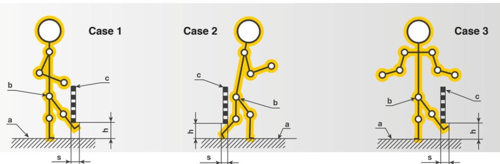
Irregular openings and accessibility from below: Slit openings >180mm and square or circular openings, >240mm allow access to the entire body.
